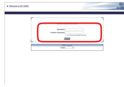
\* The login password configuration page is displayed only when EX-150AH has the factory default settings. Once configured, it will not be displayed again.
