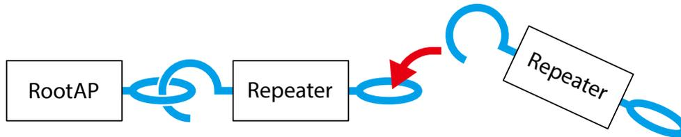
Even when connecting multiple Repeater APs to one AP-800AN unit, connect them starting from RootAP.
