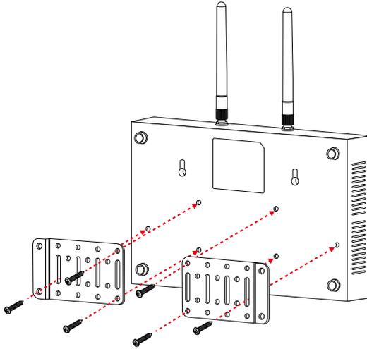
2. After attaching the bracket to AP-800AX, hold it to the wall and mark the positions of the four screw holes. Drill a pilot hole at the marked positions on the wall and insert the anchors.
