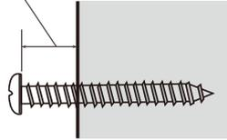
3. To mount AP-800AX to the wall, align the screws of the wall with the screw holes of AP-800AX and move the unit down along the wall to fix it.
